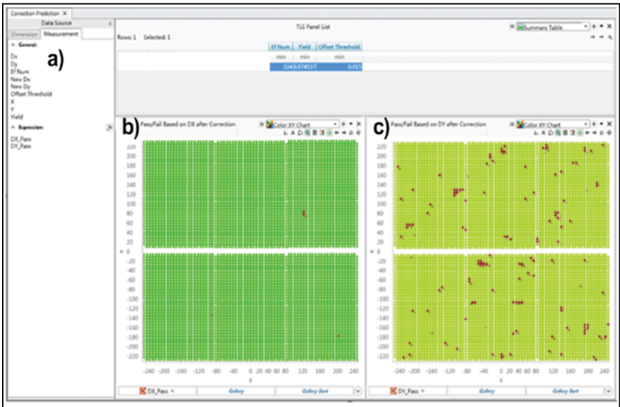
Figure 9: Visual charts and analytical tools of yield prediction technology showing: a) Various parameters for in-depth analysis; b) X-axis overlay error heat map; c) Y-axis overlay error heat map. A comparison of these maps reveals that the Y-axis exhibits the most significant overlay errors, which directly contribute to yield loss. This insight enables users to pinpoint the root cause of the issue and take corrective actions effectively, thereby improving overall process performance.
