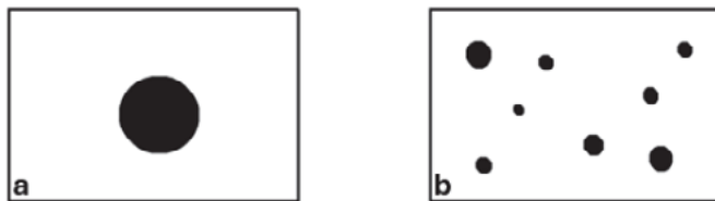
Figure 3: Example of die-attach solder void patterns used for thermal simulation of the clip-bonded package: a) 10% single large void; b) 10% multiple smaller voids.
