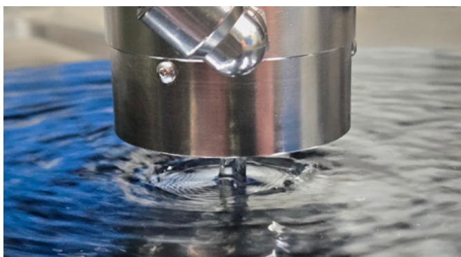
Figure 5: SpinSAM™ transducer technology: Inspecting a wafer.
