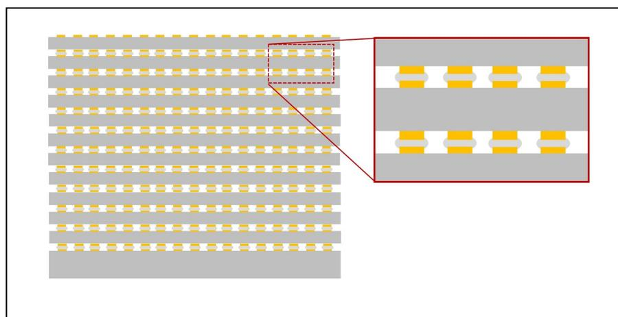
**Figure 3:** Cross-section of the next-generation HBM with flux-TCB.
