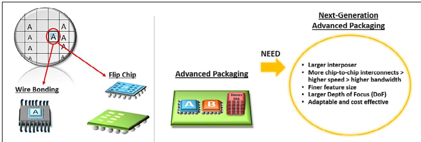
**Figure 3:** The evolution of advanced packaging to next-generation advanced packaging. SOURCE: Multibeam Corporation
