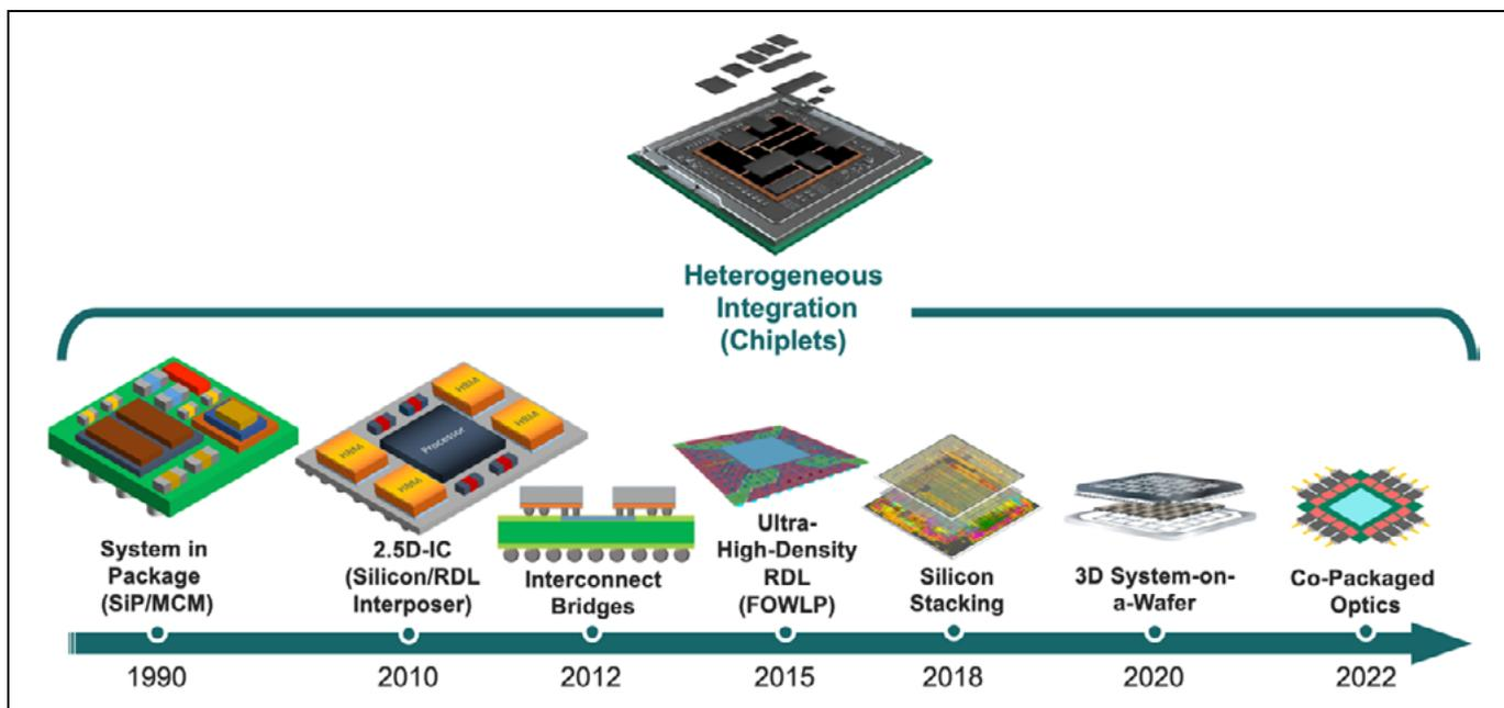
**Figure 2:** Heterogeneous integration leverages multiple packaging technologies.
