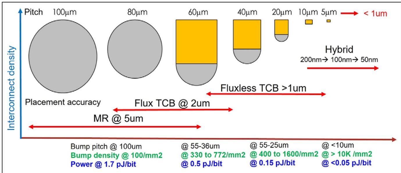
Figure 1: First-level interconnect (FLI) process mapping.
