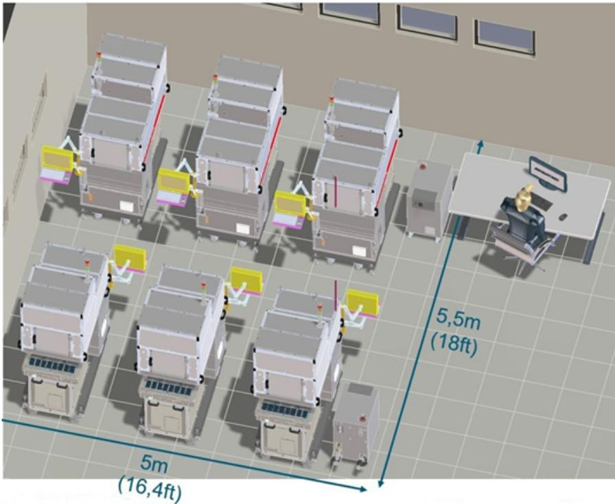
**Figure 1:** Six EX Test Stations with M4127 handlers fitting within a 5m by 5.5m laboratory space to speed up test-pattern validation and other engineering tasks.
