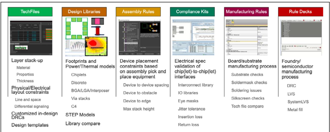
Figure 4: Package assembly design kits (ADKs).
