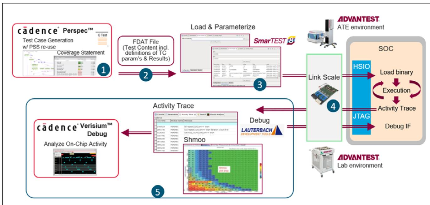
**Figure 2:** PSS enables the interfacing of EDA and ATE domains.
