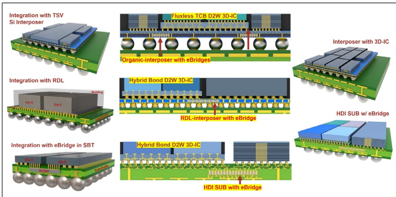
**Figure 2:** Various heterogeneous integration (HI) package architectures at a glance. SOURCE: ASMPT
