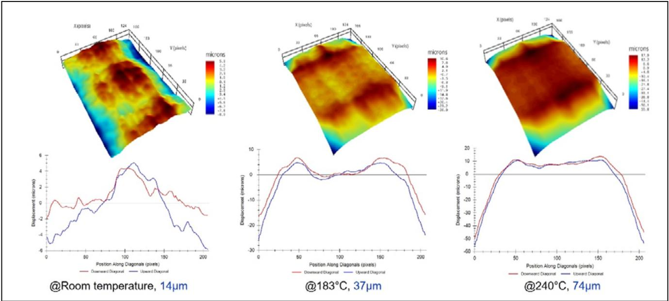
**Figure 4:** HI die warpage characterization. An example of warpage in large compound HI dies from room temperature to reflow temperature. SOURCE: ASMPT
