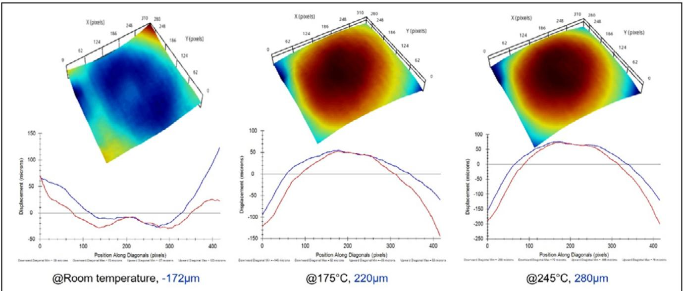
**Figure 5:** HDI substrate warpage characterization. An example of warpage in a large HDI substrate from room temperature to reflow temperature. SOURCE: ASMPT
