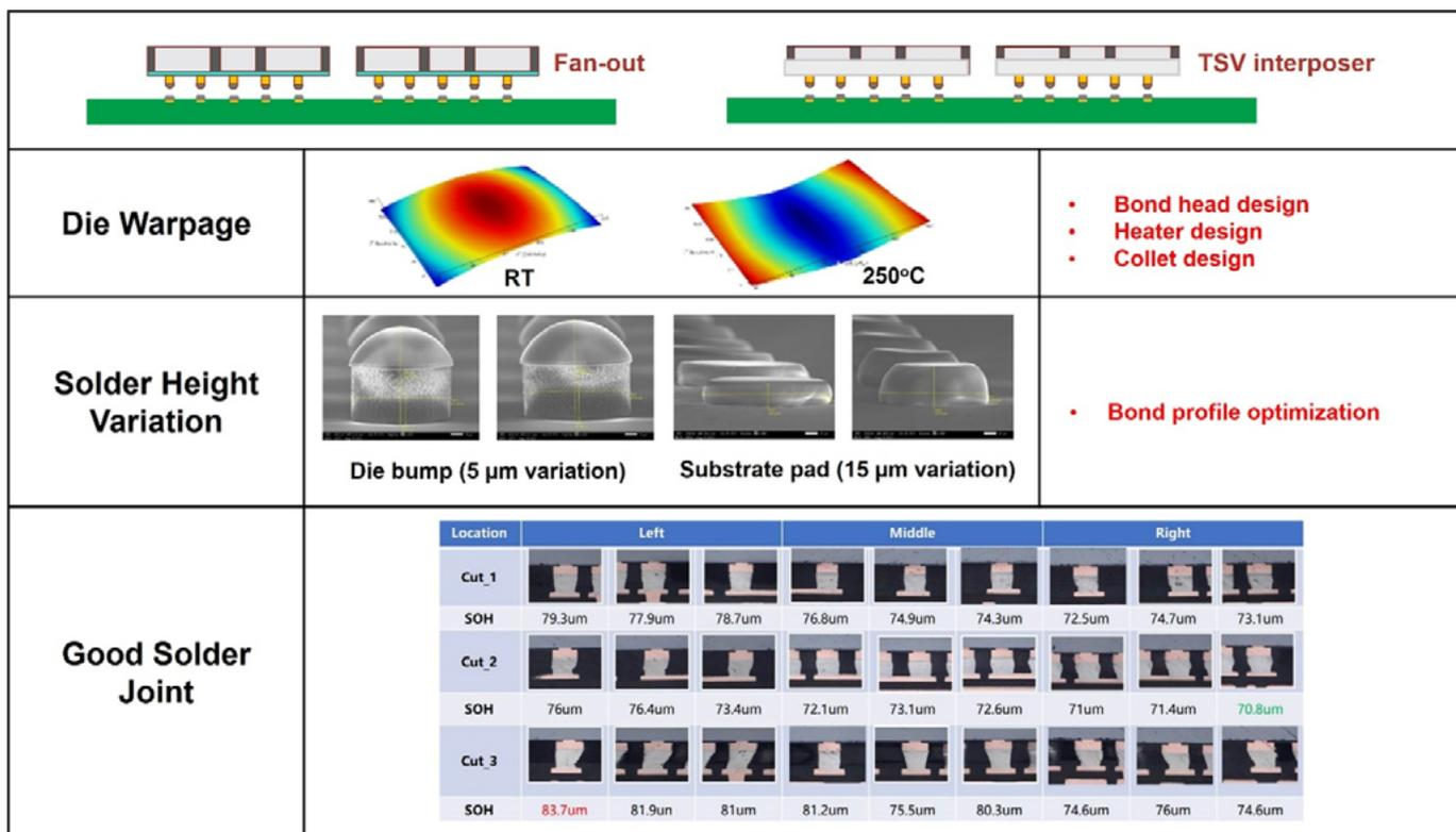
Figure 7: Challenges for extra-large HI die bonding. SOURCE: ASMPT
