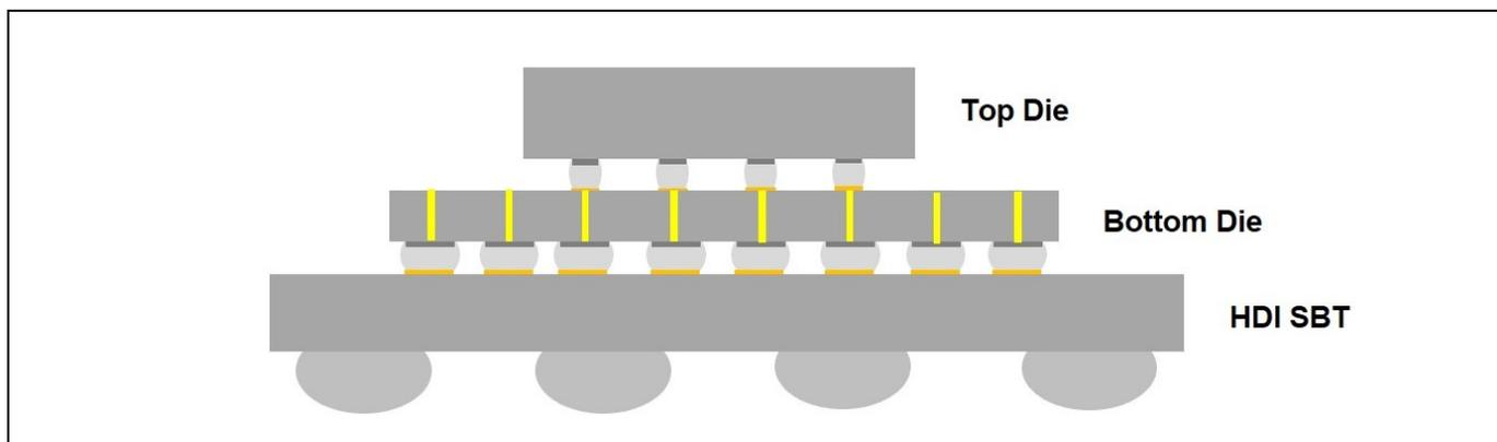
Figure 9: Fluxless bonding for 2-layer stack packages. SOURCE: ASMPT
