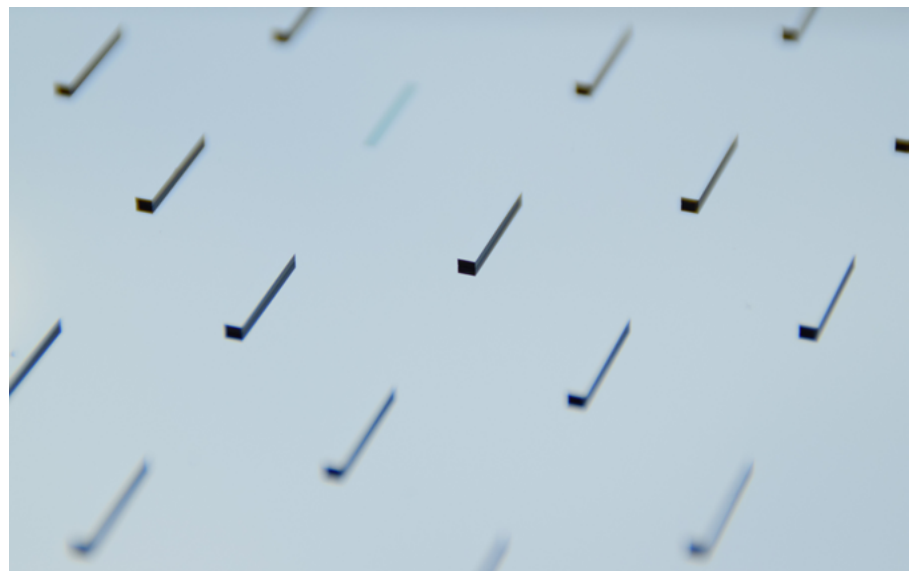
Figure 5: Self-assembly process applied to high aspect ratio dies.
