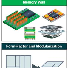
Integration in the vertical dimension/ silicon stacking technologies allows designers to potentially cram more functionality into smaller form factors while improving performance and reducing costs. Silicon stacking architectures can integrate multiple homogeneous and heterogeneous die/ chiplets, such as logic, memory, analog, and RF, into a single design. These heterogeneous, multi-chiplet architectures can provide a much lower-cost alternative to using advanced nodes (scaling).
