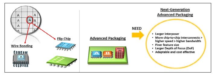
Figure 3: The evolution of advanced packaging to next-generation advanced packaging. SOURCE: Multibeam Corporation
