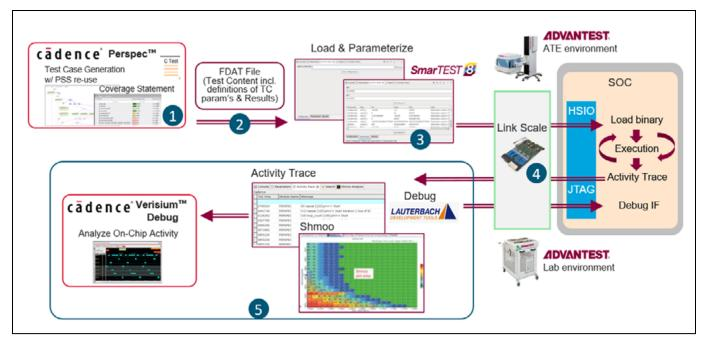
Figure 2: PSS enables the interfacing of EDA and ATE domains.
