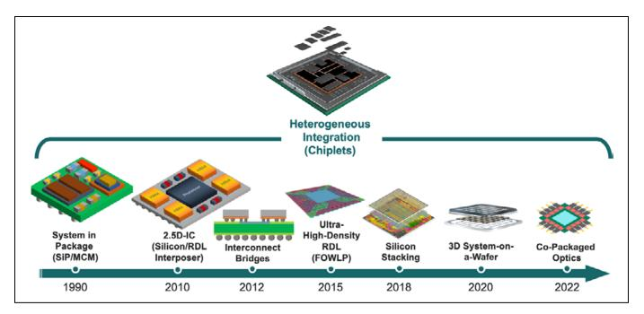
Figure 2: Heterogeneous integration leverages multiple packaging technologies.
