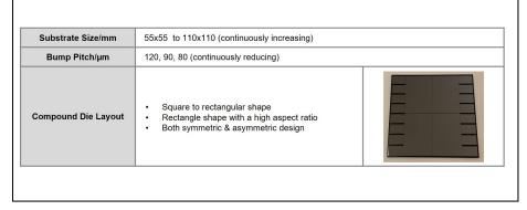
Figure 6: HI packaging architecture associated challenges and solutions with ASMPT home-built TV with 70 x 70 integrated die size.
