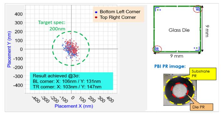
Figure 11: Alignment accuracy verification test based on COG (chip-on-glass) done on an ASMPT LithoBolt Bonder showed that a <200nm result has been achieved.
