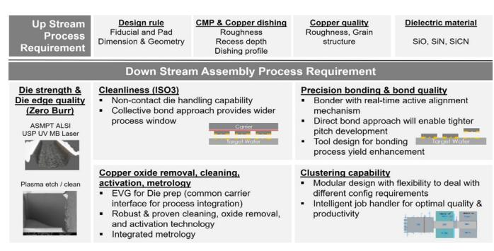
Figure 10: Key challenges and solutions in D2W hybrid bonding.
