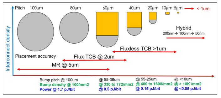
Figure 1: First-level interconnect (FLI) process mapping.
