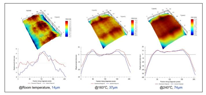
Figure 4: HI die warpage characterization. An example of warpage in large compound HI dies from room temperature to reflow temperature. SOURCE: ASMPT
