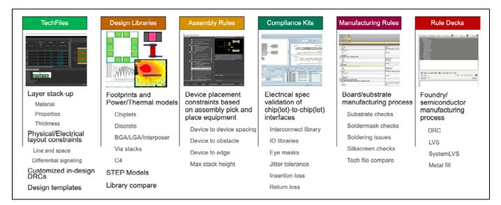
Figure 4: Package assembly design kits (ADKs).
