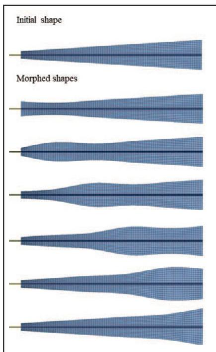
**Figure 13:** Shape perturbations used for boot geometric optimization.
