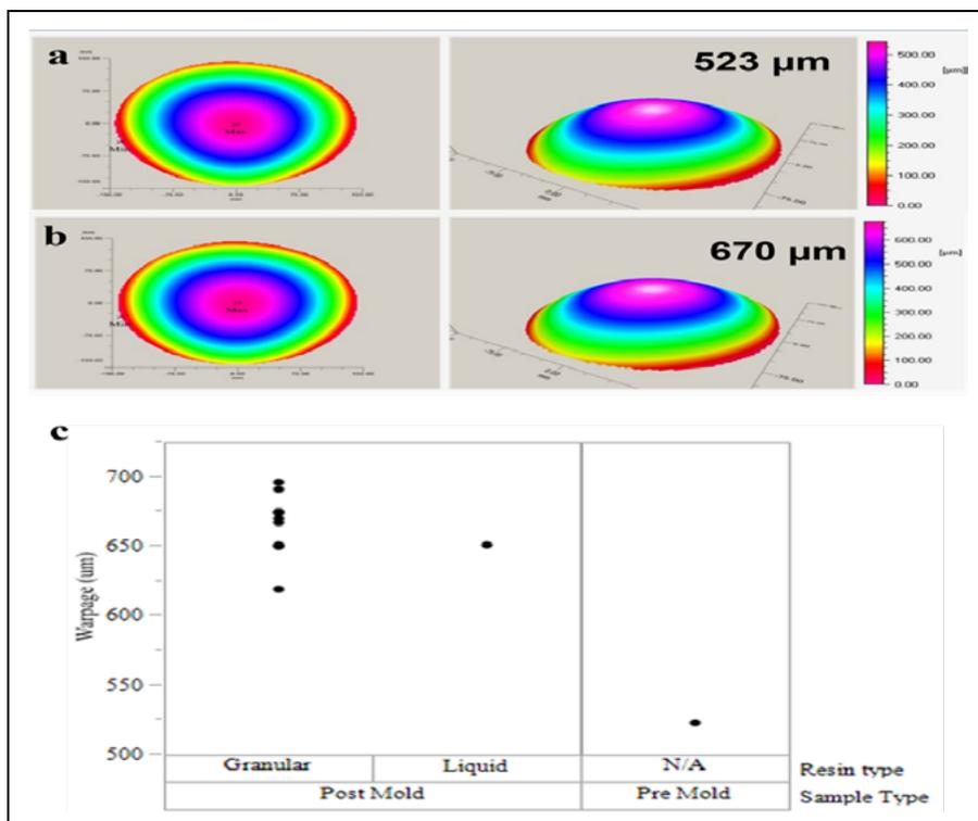
**Figure 2:** Representative 3-D warpage image for: a) pre- and b) post-mold wafers; and c) warpage value for pre- and post-mold wafers
