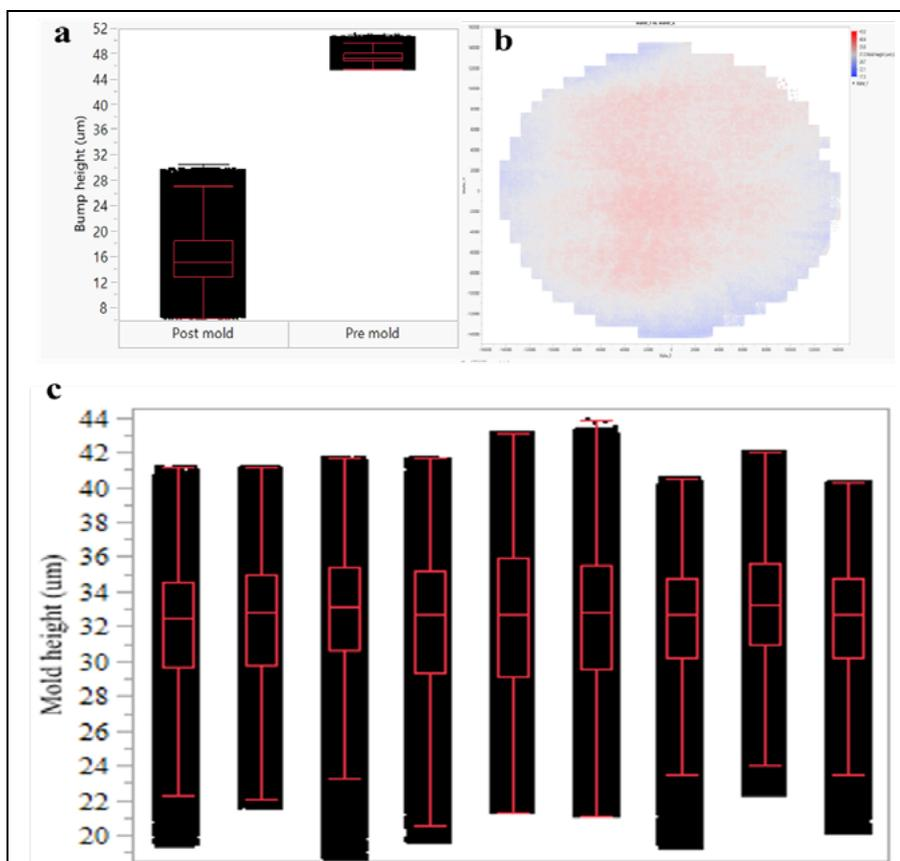
**Figure 3:** a) Bump height measurements pre- and post-mold; b) Mold height wafer map calculated from bump height measurements; c) Mold thickness distribution and range (TTV) for the different skews.
