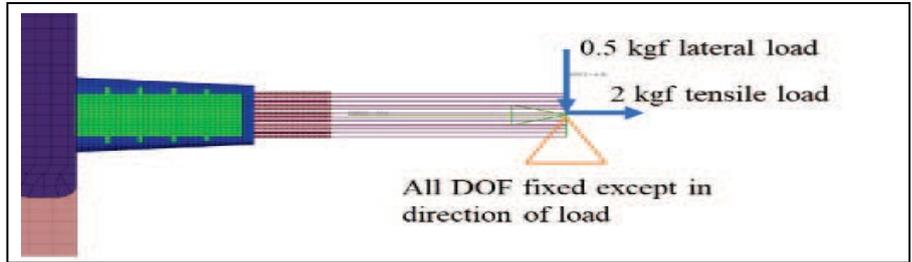
**Figure 15:** Example of loading conditions considered on the pigtail exiting the module. The tapered boot design that was included in this study is shown.
