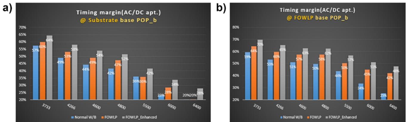
**Figure 12:** Timing margin of a PoP system for various DRAM package types with a) a substrate-based AP package, and b) a FOWLP-based AP package.
