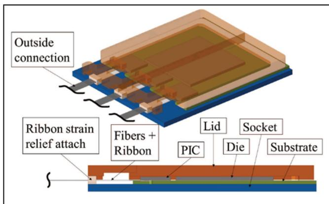
**Figure 2:** Photonic device with three pigtail ribbons exiting the module; also shown is the ribbon strain relief between the lid and substrate.
