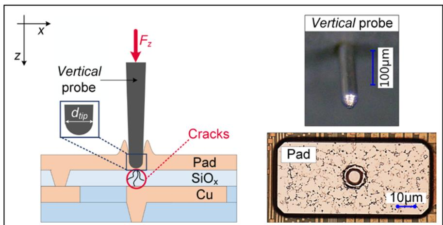
Figure 2: Vertical probe contacting a POAA, thereby inducing oxide cracks [2].
