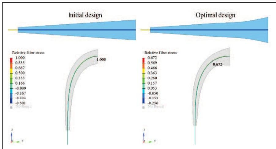
**Figure 14:** Morphologic optimization of the tapered boot. The initial and optimal shapes for such a boot are presented along with the resulting fiber stress in the side pull test load application. The shape did reduce by 33% the stress in the fiber used in our model.
