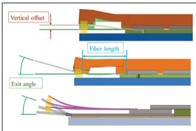
**Figure 4:** Illustration of the geometric parameters for lid and stiffener configurations; deformations were exaggerated for clarity. Anchoring outside of the package is also considered to evaluate extended fiber length.
