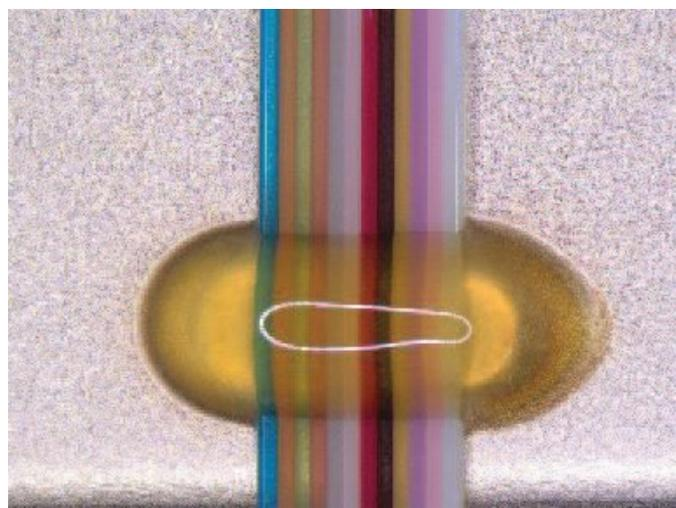
**Figure 8:** Example of ribbon attach with an adhesive on a metal-plated finish. The adhesion to the ribbon is critical to guarantee satisfactory results for the pigtail's retention tests.
