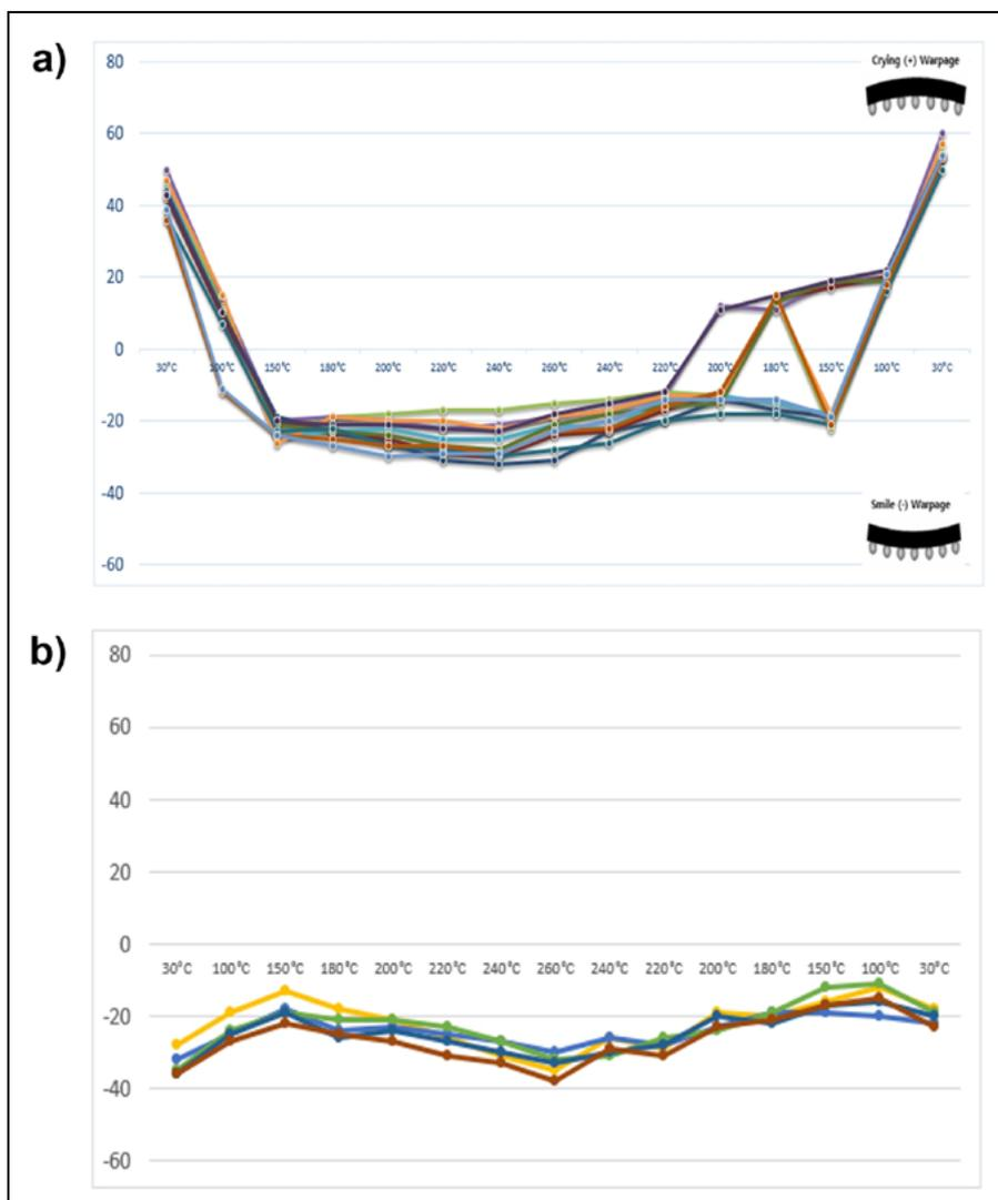
Figure 7: Warpage of a) a W/B package, and of b) a HIFOM package.
