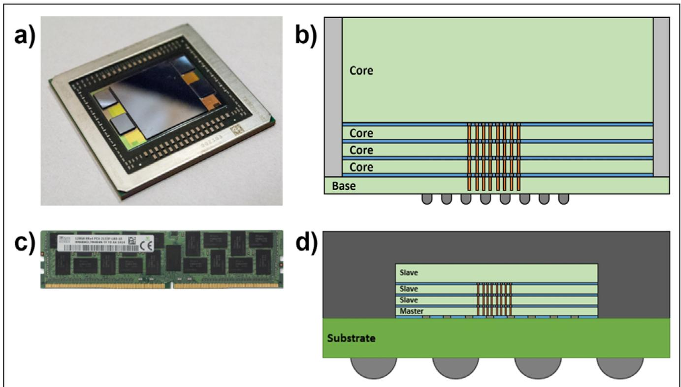
**Figure 1:** Memory applications using TSVs: a) 2.5D system in package (SiP) with HBM; b) schematic of a HBM known-good stacked die (KGSD); c) a 3DS memory module; and d) a schematic of a 3DS package.
