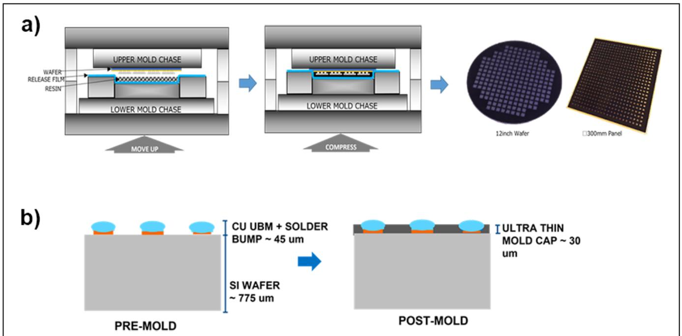
Figure 1: a) Stepwise compression molding at the wafer or panel level; b) Wafer stack with thin mold cap and exposed solder balls pre- and post-mold.
