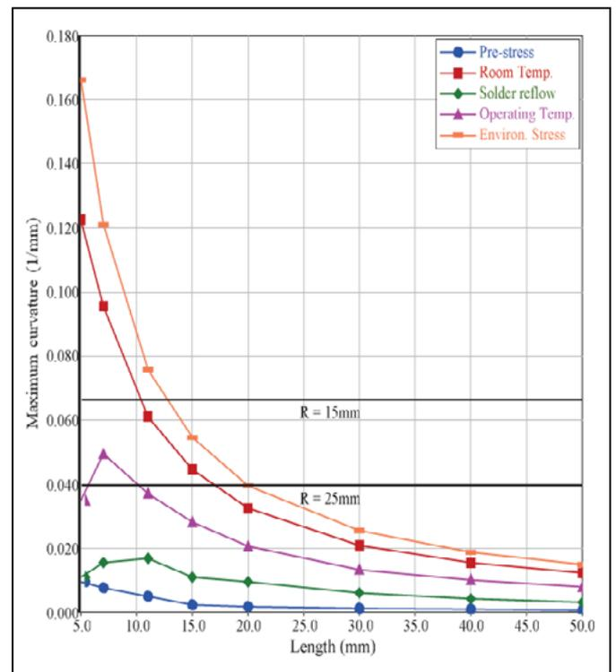
**Figure 10:** Maximum fiber curvature of various fiber free lengths of the pigtail latching within the module.
