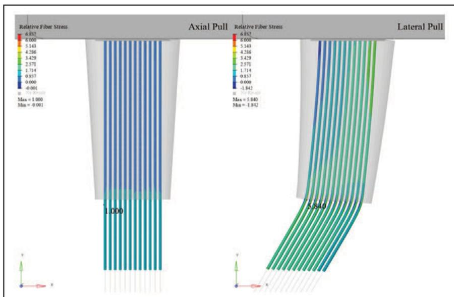
**Figure 16:** Stress comparison between the axial pull and lateral pull load cases on the tapered oval boot. The stresses from the lateral case are ~6X higher than those of the axial case.
