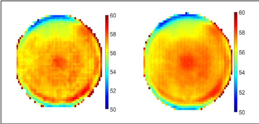
**Figure 6:** a) (left) Bump height uniformity measured with the NanoResolution MRS sensor, and b) (right) the reference confocal measurement system show consistent results. Units are in  $\mu\text{m}$ .
