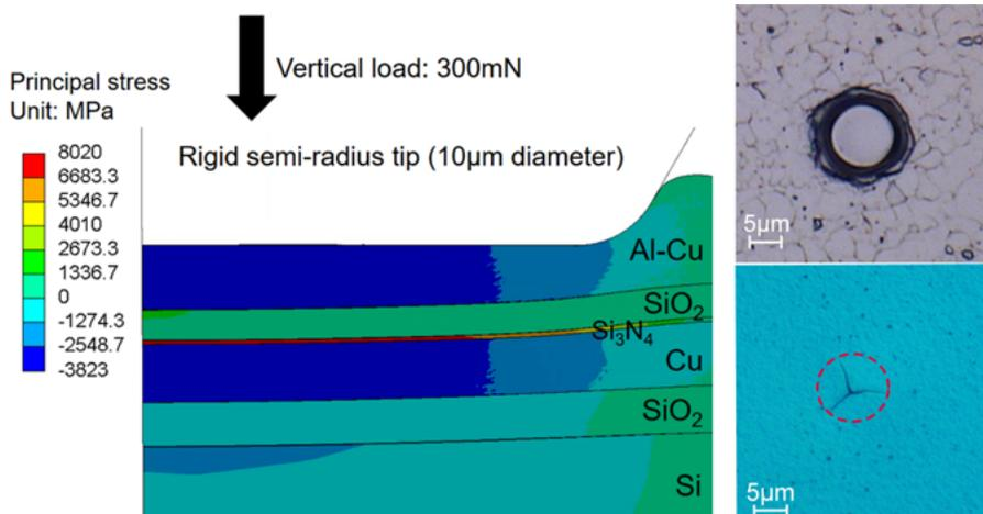
**Figure 3:** Stress in a layer stack during contacting causing oxide cracks.
