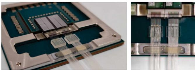
**Figure 1:** Photo of a co-package photonic module [6] with two pigtails, where the ribbon strain relief is created with adhesive on the package stiffener.
