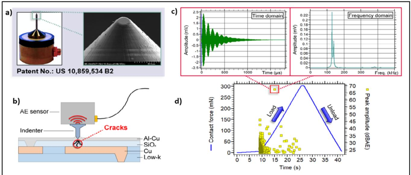
**Figure 5:** a) Patented sensor-indenter system; b) Crack detection by AE test method; c) Acoustic signal in time and frequency domains; and d) Typical contact cycle.
