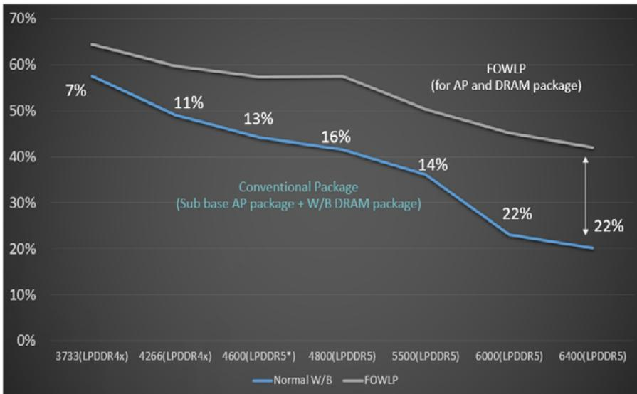
**Figure 13:** Delta of the timing margin as a function of clock speed.
