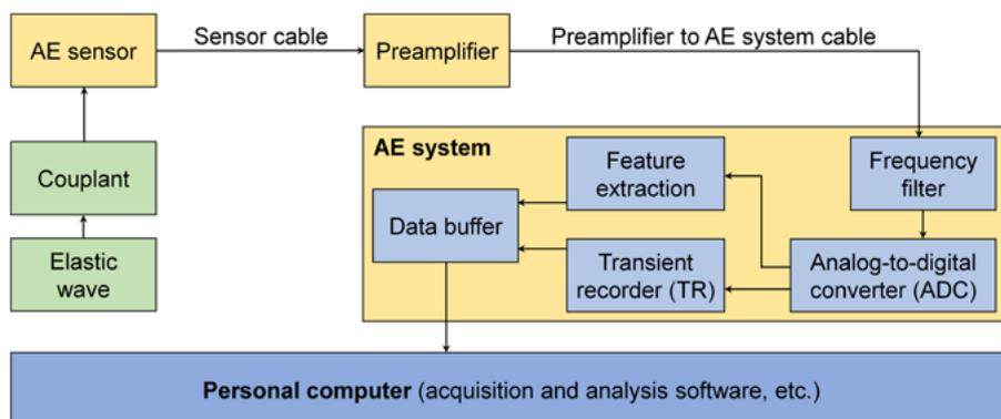
**Figure 4:** Schematic view of AE measurement chain [2].
