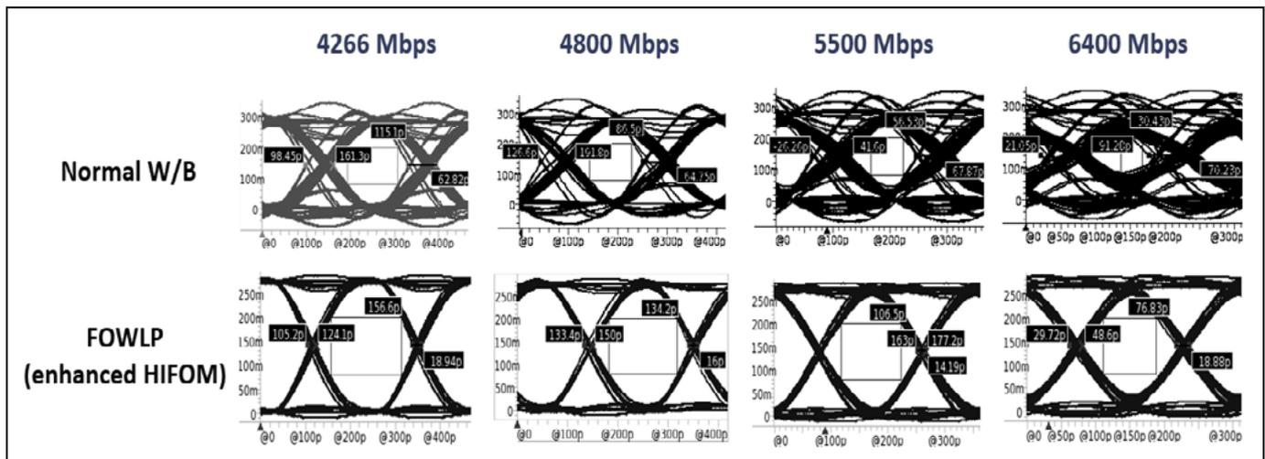
**Figure 11:** Data eye diagrams for two different packages at four different frequencies.
