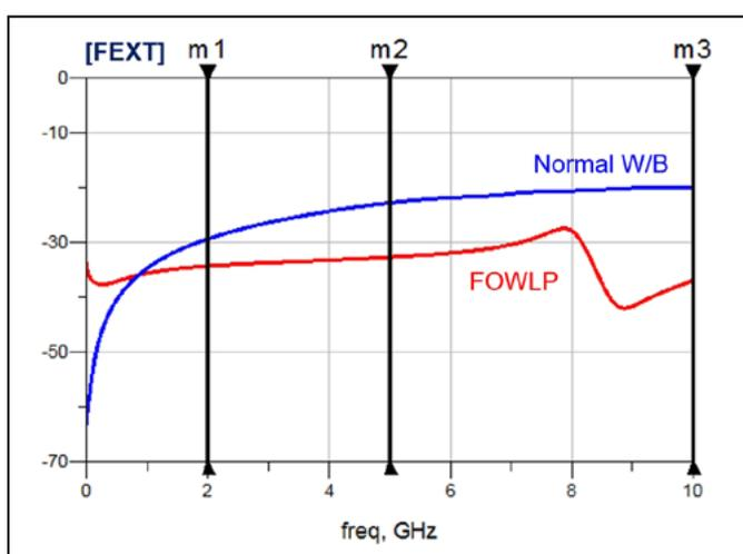
**Figure 10:** Crosstalk curves of a normal W/B package and of a FOWLPL.
