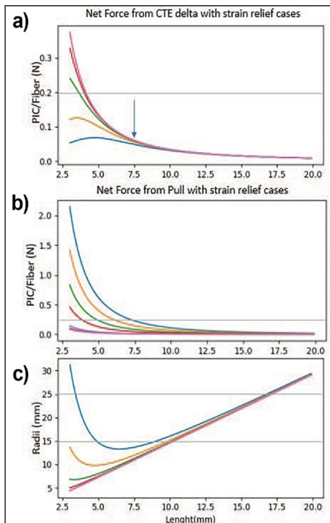
**Figure 7:** Impact on anchoring distance for various height values for: a) (top) CTE force, b) (middle) pull force; and c) (bottom) radii.
