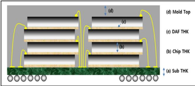
**Figure 2:** A simple representation of mobile memory packages with normal wire bonding interconnections.
