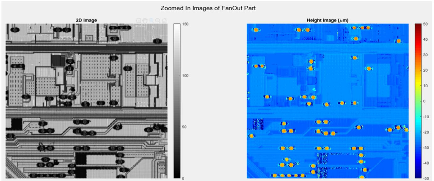
**Figure 7:** a) (left) A 2D image of fan-out patterns on a wafer; and b) (right) a merged image showing superimposed bump height data.
