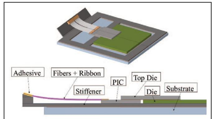
**Figure 3:** Photonic device with pigtail strain relief is the attachment on the module's stiffener.
