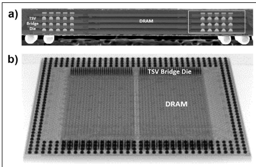
Figure 6: a) Cross sectioned and b) X-ray images of a HIFOM package.
