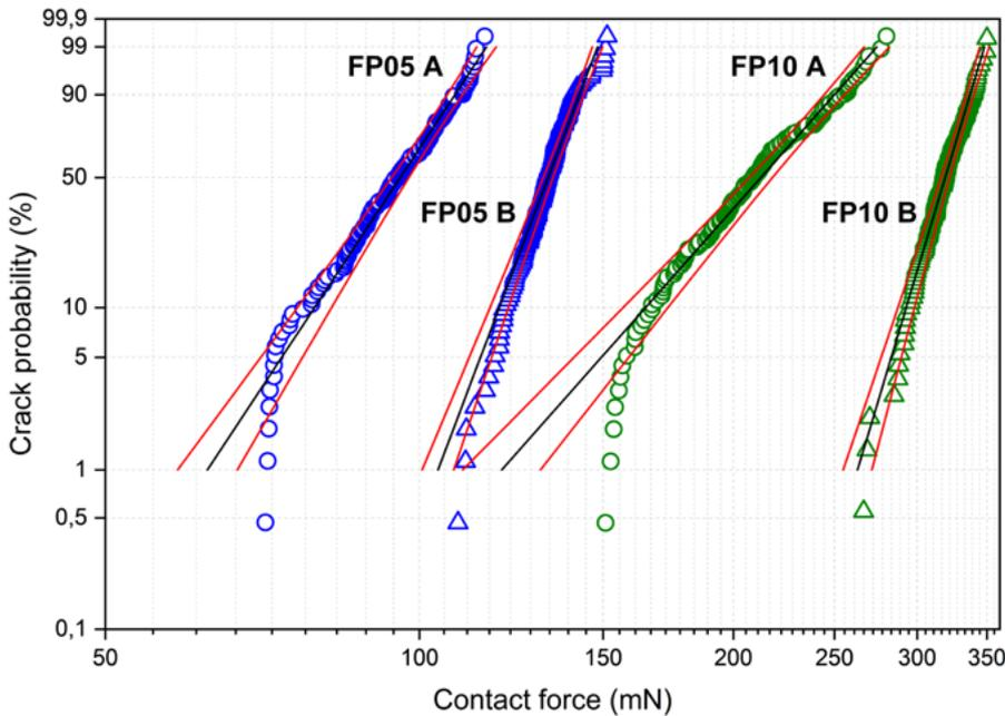
**Figure 9:** Crack probability plot for pad stack option A vs. B and tip diameter  $5\mu\text{m}$  vs.  $10\mu\text{m}$  on the Weibull scale.
