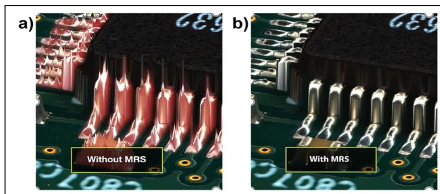
**Figure 4:** Imaging a) without and b) with multi-reflection suppression technology<sup>®</sup>.
