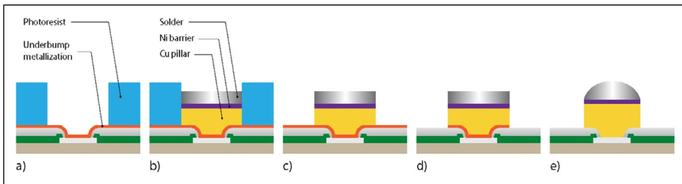
**Figure 2:** Copper pillar bump process flow. Conventional bump height measurement is done after photoresist stripping; a) before bumping; b) bump plating; c) photoresist strip; d) UBM etching; e) solder reflow.
