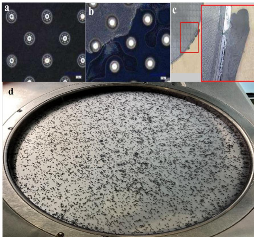
**Figure 5:** a) Bump mold encapsulation at center; b) the edge of an incomplete filled wafer; c) resin bleed-out at the edge of the wafer; and d) granular resin distribution on the bottom chase pre-compression molding.
