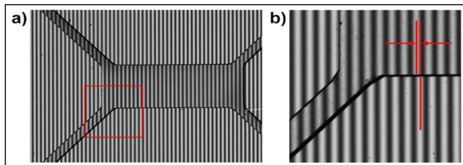
**Figure 3:** The projected fringe pattern is distorted (shifted) wherever the height of the imaged object changes; a) (left) The VLSI step standard in this example is a recessed rectangular feature on a flat background; b) (right) A close-up of one corner shows the phase shift, indicated by the red arrows, more clearly.
