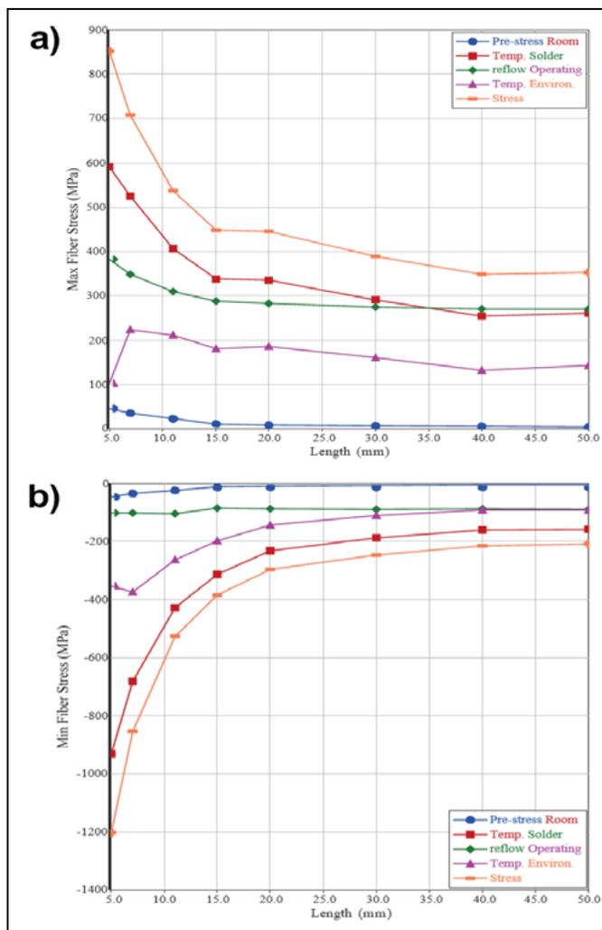
**Figure 9:** a) Maximum and b) minimum fiber stresses vs. the fiber free length for the pigtail configuration.
