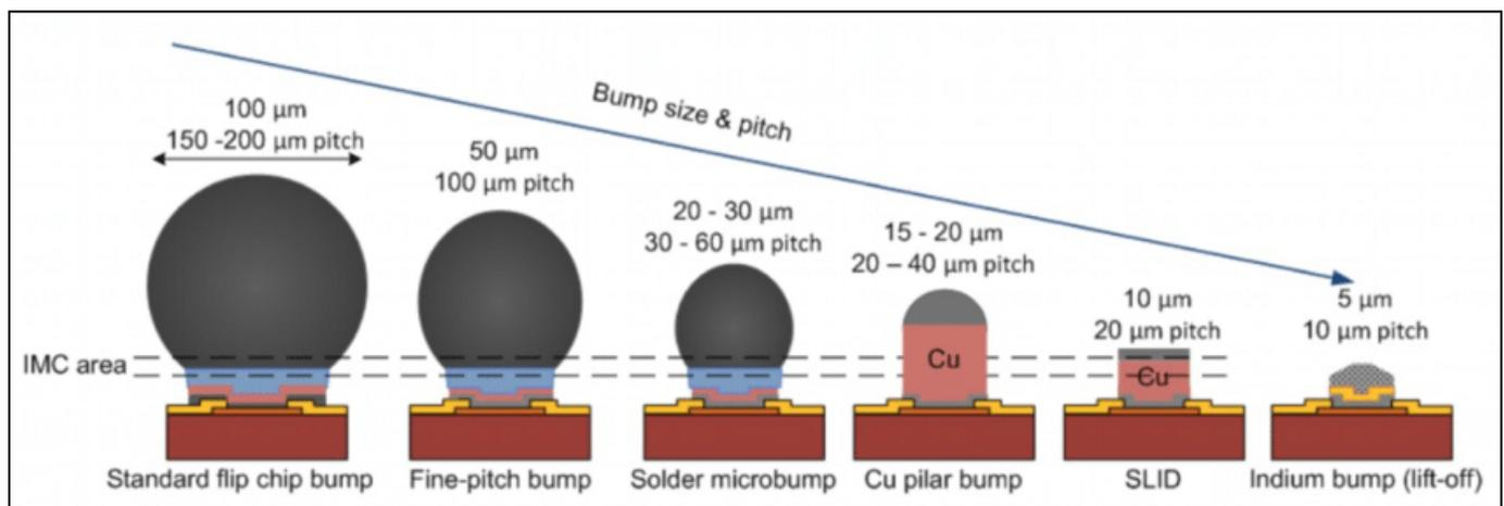
**Figure 1:** Evolution of bump size and pitch. Image courtesy of T. Tick and S. Vahanen [1]
