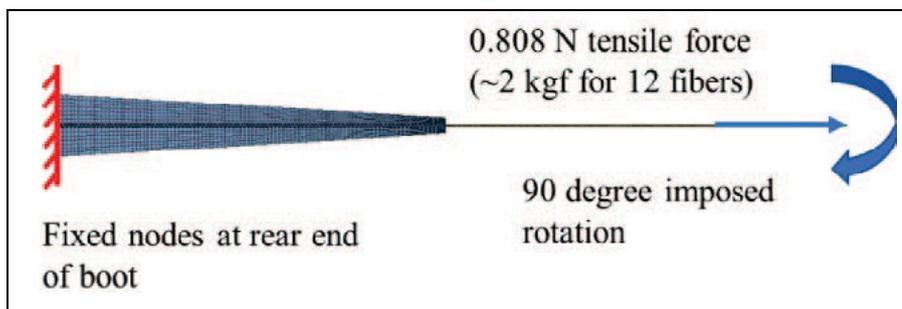
**Figure 12:** Description of the loading conditions used for boot optimization.
