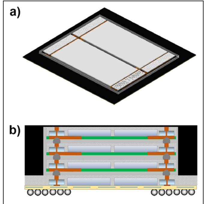
**Figure 4:** Schematic illustration of a HIFOM a) floor plan, and b) cross-sectional diagram.
