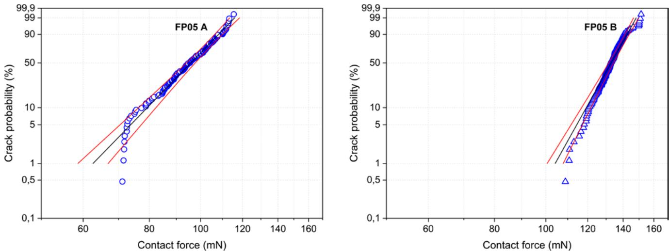
**Figure 8:** Crack probability plot for: a) (left) pad stack option A vs. b) (right) B and tip diameter 5µm on the Weibull scale.
