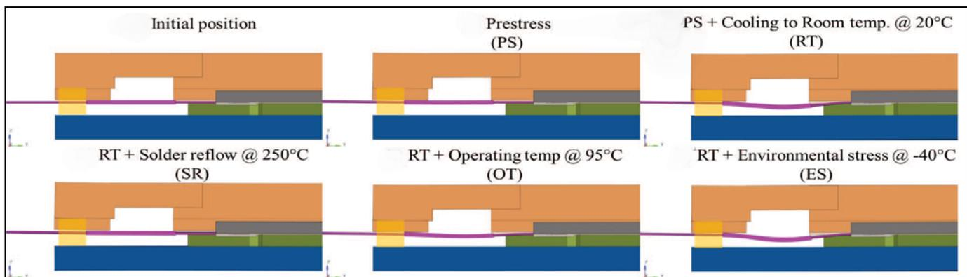
**Figure 6:** Illustration of the module geometry after the various assembly steps and loading conditions, where an S-bend in the fibers is present at temperatures below the adhesive cure.
