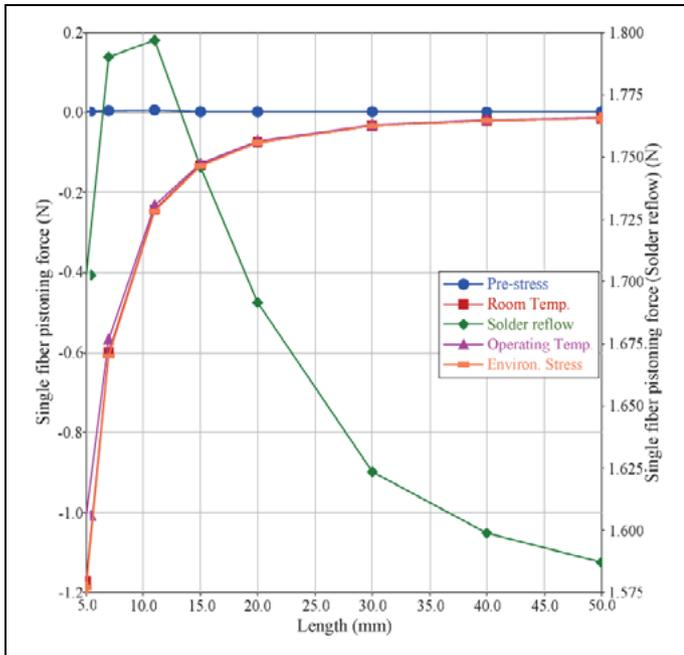
**Figure 11:** Fiber pistoning force for various fiber free lengths secured inside the package of the pigtail fiber ribbons. The solder reflow load case is read along the right axis. As the length is reduced, a higher pistoning force is measured on the V-groove because there is less bending to accept the various strains induced by the load cases.
