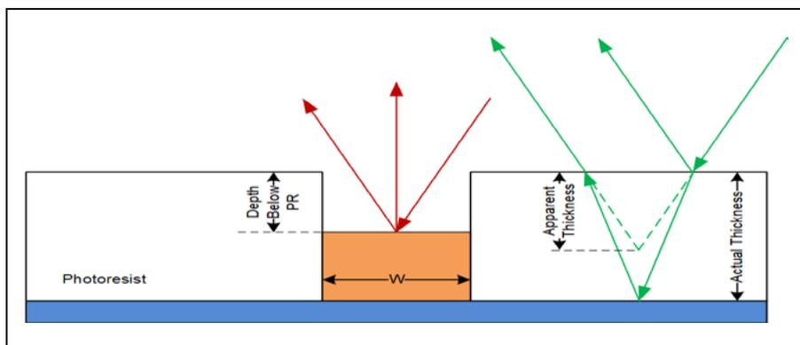
**Figure 5:** Measurement of bump height before photoresist stripping, using light refracted through the photoresist to determine the photoresist thickness and calculate bump height above the wafer surface.
