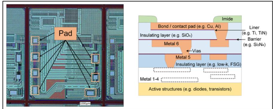
Figure 1: POAA layout for a) (left) CMOS chip design, and b) (right) a schematic cross-section view [2].
