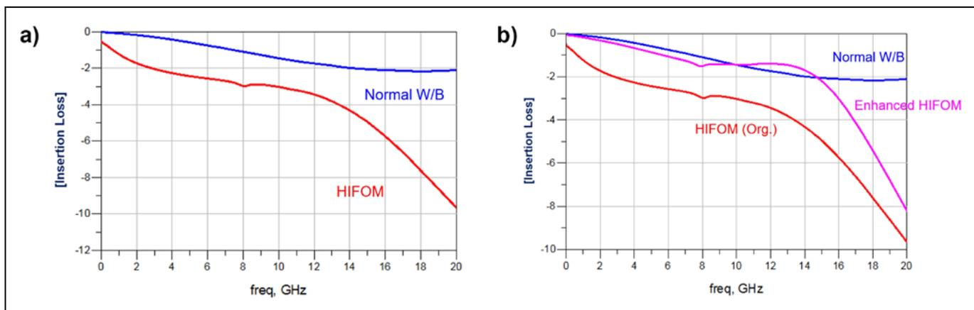
**Figure 8:** Insertion losses of a) W/B and HIFOM packages, and of b) an enhanced HIFOM package.
