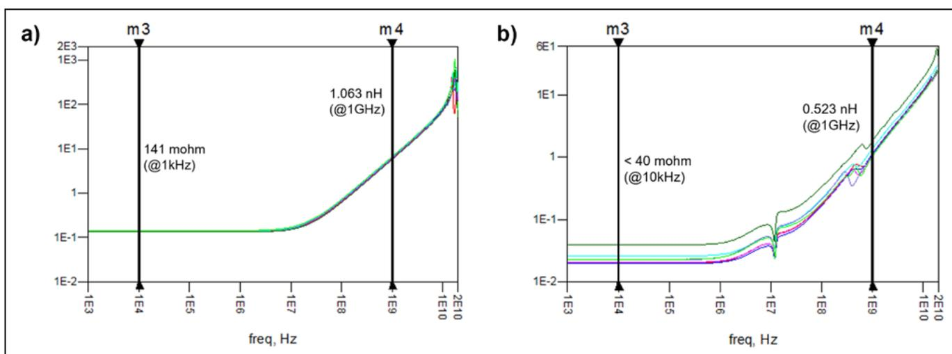
**Figure 9:** PDN impedances of a) a W/B package and b) a FOWLPL.
