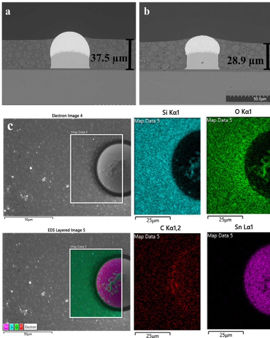
**Figure 4:** Mold height at the a) center and b) edge of the wafer; c) SEM microscopy and EDX profile showing solder ball encapsulated by mold material all around. The center and edge both showed comparable encapsulation and minimal contamination.
