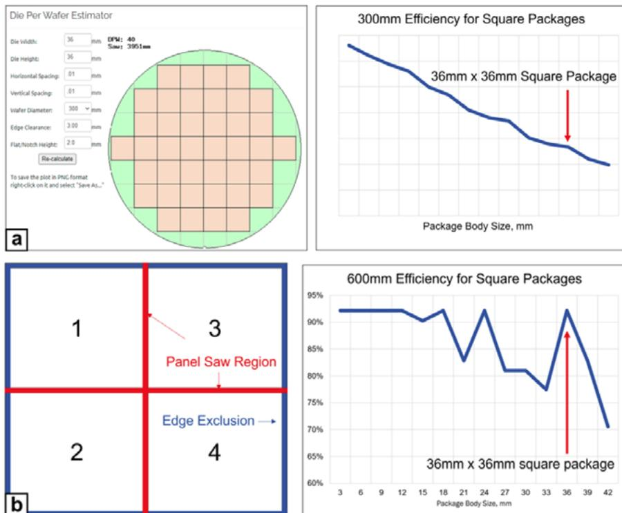
**Figure 2:** Format efficiency of: a) a 300mm round wafer, and b) a 600mm large panel for a 36mm x 36mm square package.
