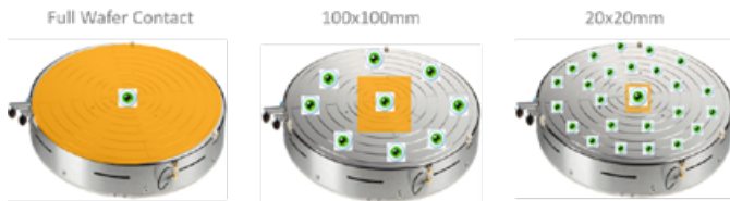
Figure 2: Number of sensors scaled to contact area size, ordered from low- to high-sensor array density.
