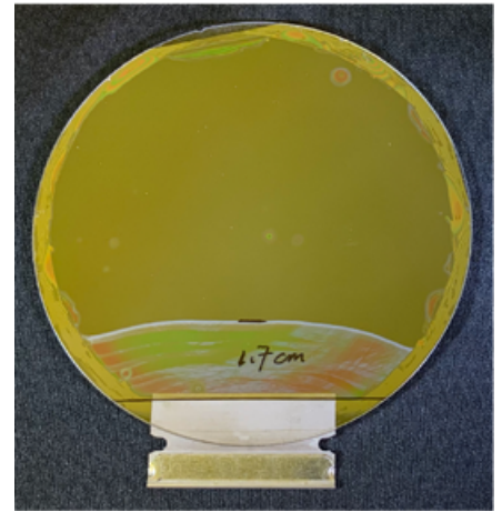
Figure 6: Wafer-level Maszara bond strength test.
