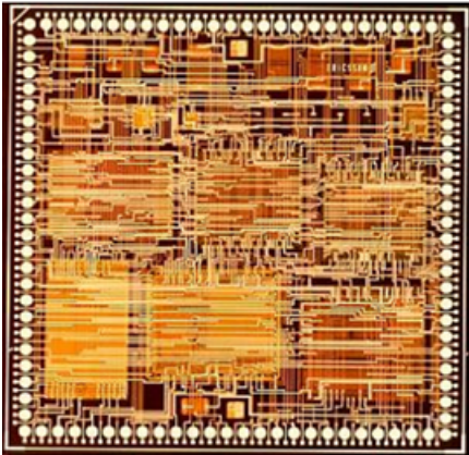
Figure 9: Mixed analog/digital COF module with embedded chips and passive devices.
