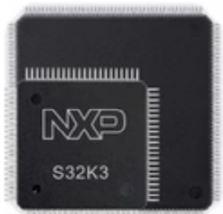
Figure 4: A visual comparison between the 172-lead MaxQFP (16x16mm) and the 176-lead QFP (24x24mm) showing the body size reduction of 55%.
