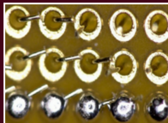
Through Hole Technology Soldering
