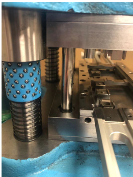
Figure 2: The manual trim and form tool used to build the first MaxQFP samples by hand.
