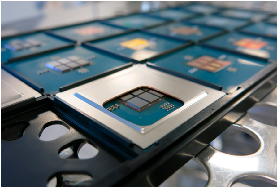
Figure 4: IntAct interposer. © CEA-Leti
