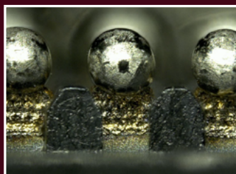
Presoldering of SMD Connector Elements
