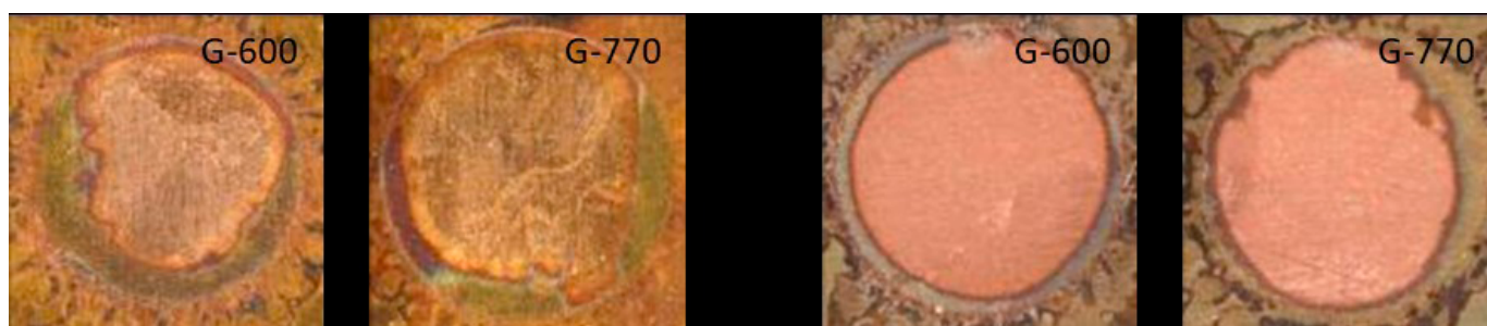
Figure 3: Alloy surface after MSL-1, reflow, and button shear—untreated on the left, treated on the right.
